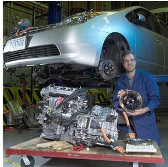
**CTR researcher Ted Bohn holds the new engine torque sensor installed in Argonne's 2004 Prius. With this new design, no vehicle modifications are required, saving almost \$20k in custom brackets and vehicle work.**
