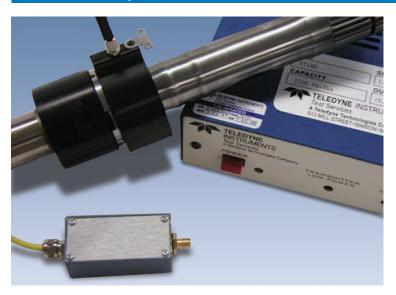
CV shaft torque is often difficult to obtain because of limited space in this very hostile under-vehicle environment. The AT100 uses non-contact, digital data transfer technology to provide the user with a clean and responsive torque signal. Power is inductively supplied to the rotating collar eliminating the need for batteries.
